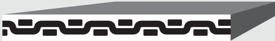
Reinforcement threads are crimped
